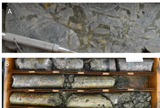
Figure 5: Examples of late-stage mineralization styles: A) Glory Hole breccia with pyrite-chalcopyrite cementing angular, sericite-kaolinite altered clasts. B) Massive chalcopyrite-bornite-pyrite mineralization from Copper Prince. The overall zone has 10.83% Cu over 15 m.
