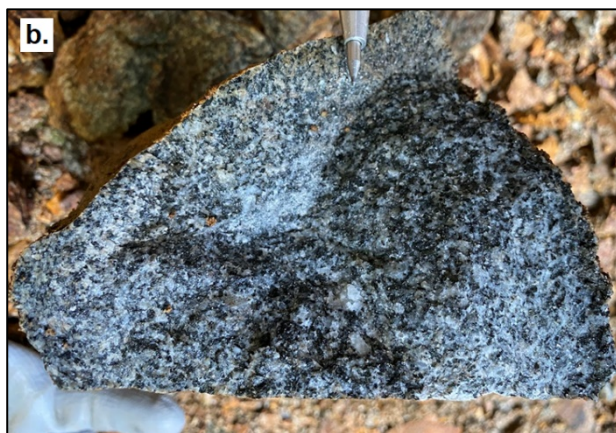
Figure 2. Main intrusions in the Tres Cerrillos prospect. a. Syn-mineralization, quartzdioritic porphyritic intrusion, showing sericitic alteration with D-type veins. b. Unaltered, equigranular, phaneritic granodiorite (precursor intrusion).
