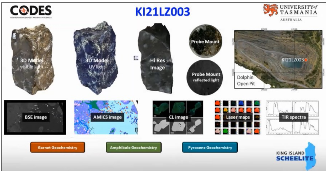
Figure 5. Illustration of Information types available for sample K12LZ003 from the Dolphin tungsten deposit, including: visible light, ultra violet (UV) light, high resolution imagery, back-scattered electron (BSE), SEM-based automated mineral classification (AMICS), cathode luminescence (CL), and hyperspectral (TIR = thermal infra-red). Buttons at the bottom show links to geochemical data available for specific minerals.
