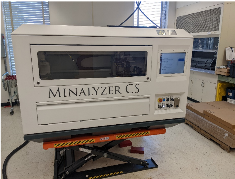
Figure 1. The Minalyzer continuous X-ray fluorescence (XRF) core scanner at Colorado School of Mines.
